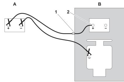
3. Inspect battery in disabled vehicle (B) for signs of cracking, bulging, leaking, or other damage. Connect red positive (+) jumper cable clamp to positive (+) post (2) of battery in disabled vehicle first.
