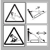
**WARNING** Tipover possible. Machine can tip over and crush you.
